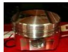
The RB25/26 spec pistons have a smaller deck height vs. RB30 pistons.
