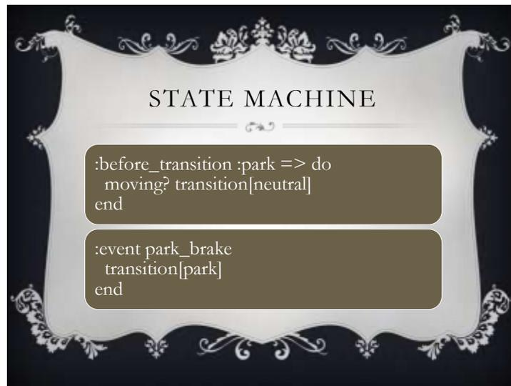
So we're heading back to our car/computer example. We want to set up a system of control for the transmission. We're going to set up an event handler to respond to pulling on the parking break to shift to park. We want to ensure that the sensor data for the vehicle in motion is compared before putting the car in park.
