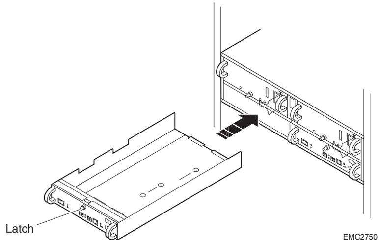
**Figure 3-12** Installing an SP (CX300 Shown)
