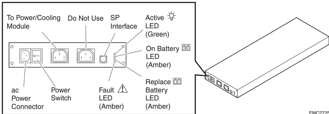
**Figure 4-1** CX300/CX300i SPS Rear Panel
