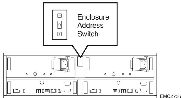
**Figure 1-4 DPE2 Enclosure Address Switch/Indicator (CX300 Shown)**
