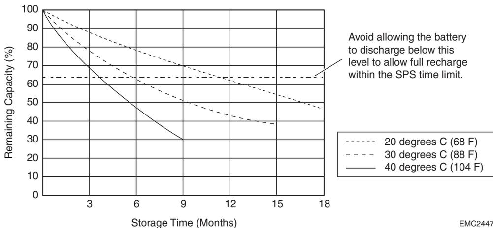
Figure A-1 Typical SPS Self-Discharge Levels at Different Storage Temperatures
