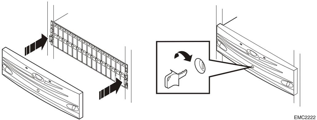
**Figure 3-10** Installing and Locking the Front Bezel
