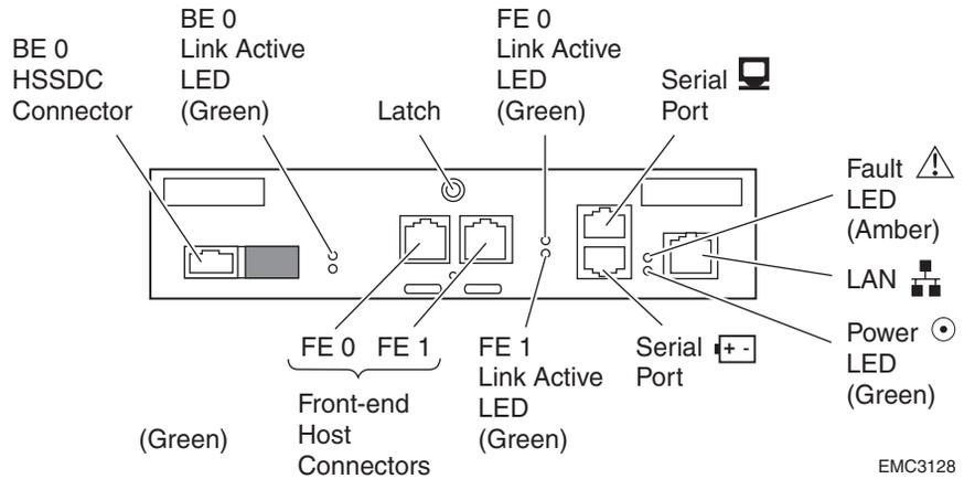
**Figure 1-7 CX300i Storage Processor**
