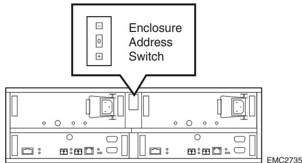
**Figure 2-1 Enclosure Address Switch (CX300 Shown)**
