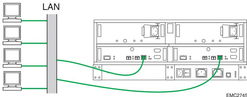
Figure 2-12 Connecting the CX300 to a Shared LAN
