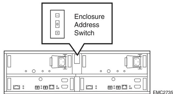
**Figure 2-1 Enclosure Address Switch (CX300 Shown)**
