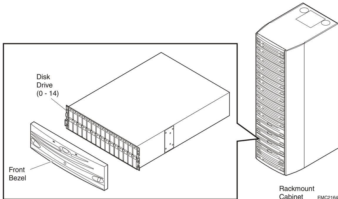
**Figure 1-1 Model CX300/CX300i Disk Processor Enclosure (DPE2)**
