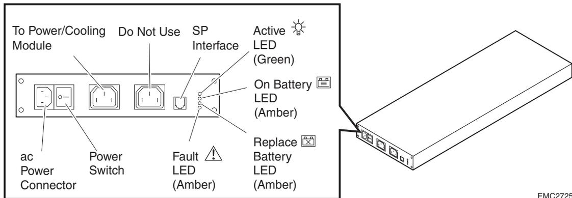
**Figure 4-1** CX300/CX300i SPS Rear Panel
