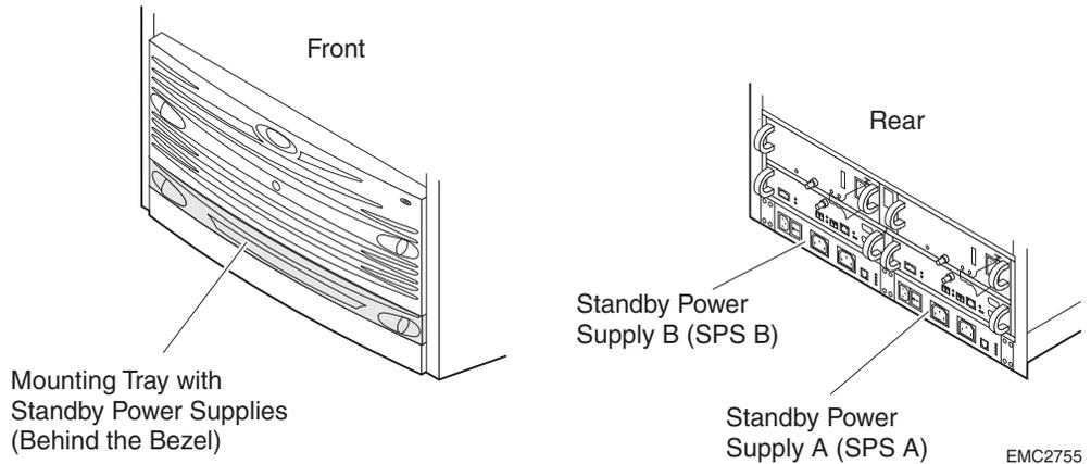
**Figure 4-2 SPS Installation, Front and Rear Views**
