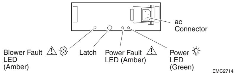
**Figure 1-9 Power Supply/System Cooling Module (ac System Shown)**
