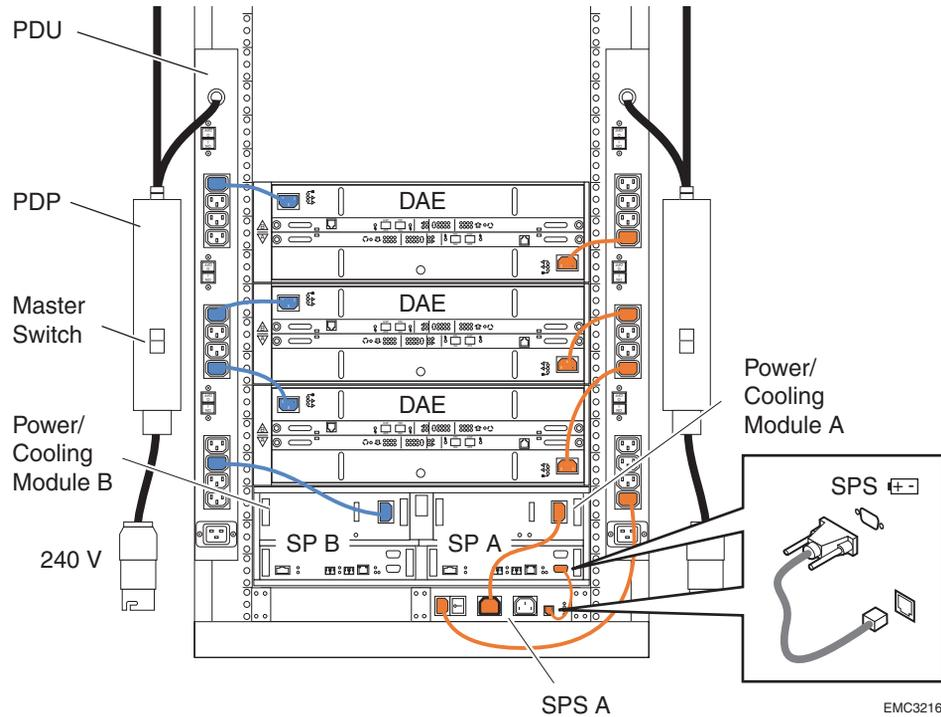
Figure 2-5 Power Connections (CX300 Shown)
