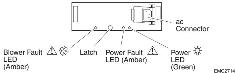
**Figure 3-2 Power Supply/System Cooling Module Status Indicators**
